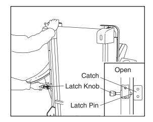
Hold the metal frame firmly with both hands, and lower it to the floor. CAUTION: To decrease the possibility of injury, do not lower the frame by gripping only the plastic foot rails. Do not drop the frame to the floor. Make sure to bend your legs and keep your back straight.
